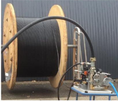
Photo 1 Cable and cable blower used in blowing test
